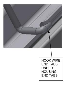
To install lens assembly guard, verify that the luminaire is completely assembled. Install lens guard on lens assembly by hooking the guard's end tabs under the luminaire housing's end tabs. Verify a tight attachment.
